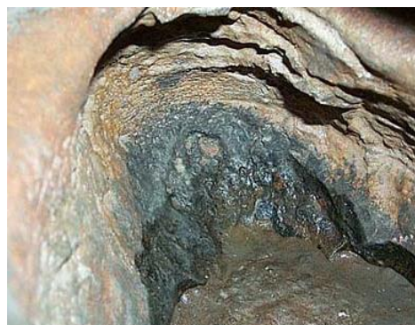
Later, this football-sized hole was found in the head of the reactor.
